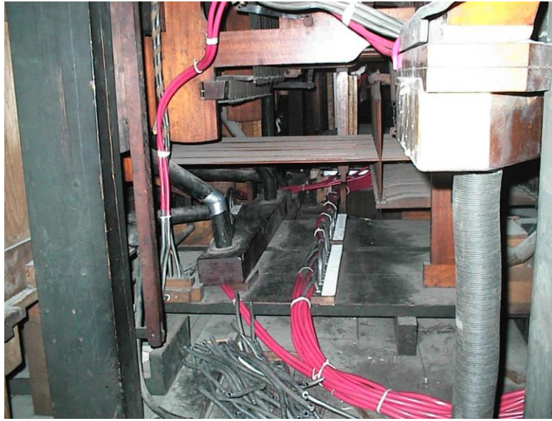
New pneumatic tubing fitted to the Pedal Organ in 2007.
