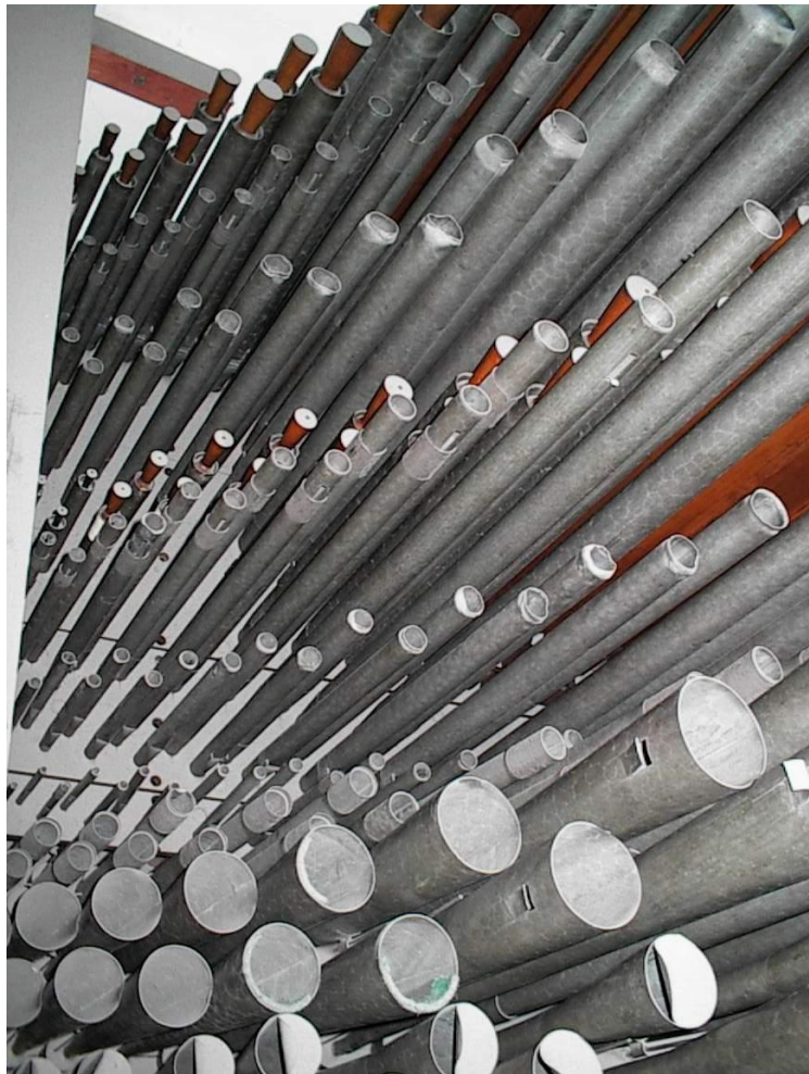
A view inside the Swell box showing the high-quality spotted metal used in Lewis organ pipes.
